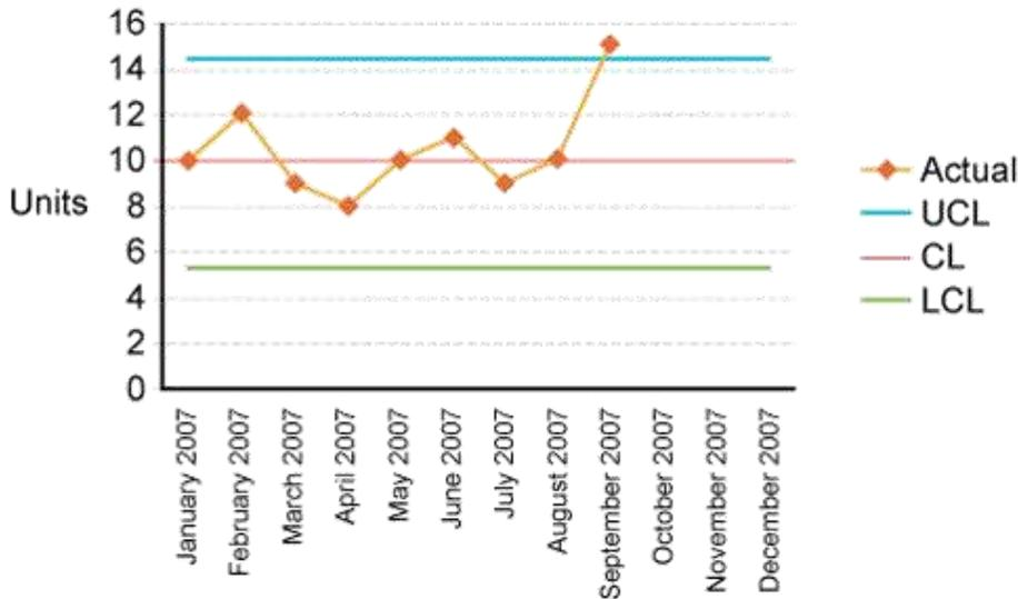
*The point at which the Actual Limit (AL) crosses the Upper Control Limit (UCL) on this chart indicates an out-of-control situation. In this case, up is bad — and the root cause must be identified and eliminated.*
